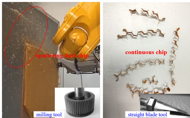
FIGURE 1. Comparison of chip formation between milling [7] and V-shaped cutting.
